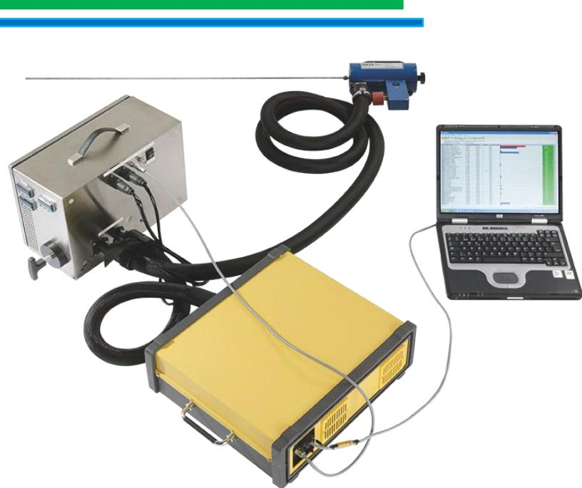
The Gasmet DX4000 is used with a standard laptop computer and Calcmet software, which provides visualization of results, IR spectra and time trends. It controls the gas analyzer and sampling unit, and has support for analog and fieldbus I/O. All measured data is stored on the laptop computer and recorded spectra can be re-analyzed later.
