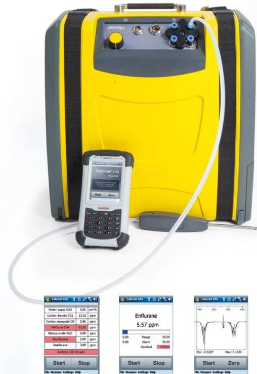
Gasmet DX4040 is standard equipped with an IP67 rated PDA and Calcmet Lite software. Large touch screen buttons and keypad are easy to use even in demanding field conditions. All measured data is stored on the PDA and can be sent as e-mail messages with the built-in 3G modem and Wireless LAN adapter.
