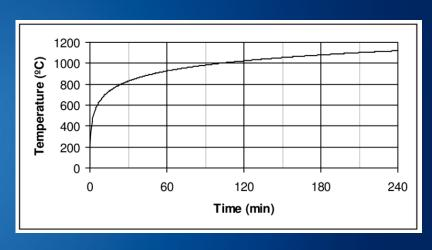
Standard time-temperature curve for an ASTM E119 fire exposure
