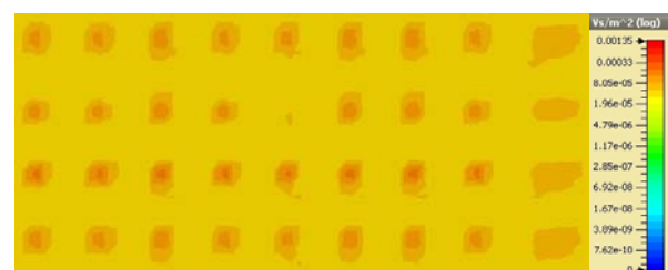
Figure 8. Magnetic flux density B[\mu\text{T}] for a sofa bed at a distance of 5cm from the mattress core along the control line
