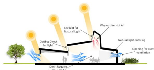
Figure 6. Diagram of integrated natural ventilation and daylighting through skylight and stack effect
