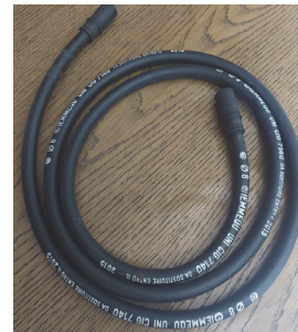
Figure 4. Marking on the hose according to the UNI 7140 standard
