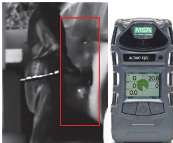
Figure 3. Vapour source identification and gas detection
