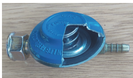
Figure 3. Gas flow regulator
