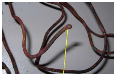
Figure 9. The copper conductor in which there is visible trace of melting as a result of the high temperature of electric arc
