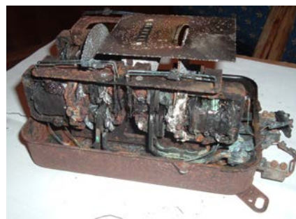
Figure 10. The appearance of the inside of a burnt-out electricity meter
