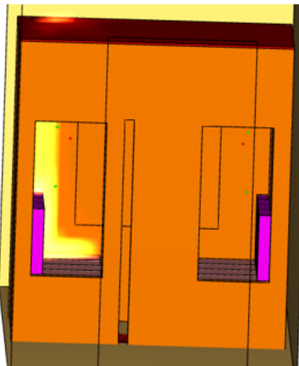
Figure 6. Fire development at 296 s
