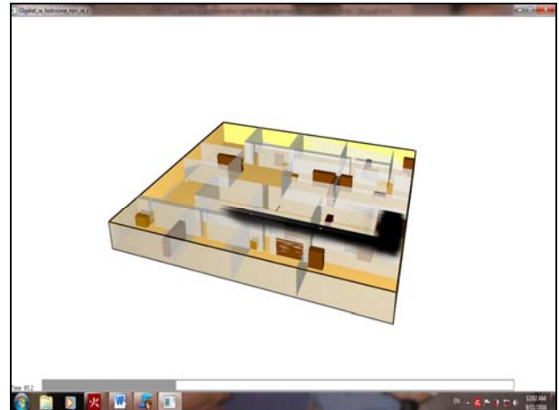
Figure 7. The presentation of the potential fire propagation after 85.2 seconds for the first case
