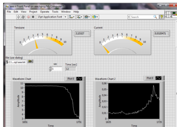
Figure 3. The front panel of the virtual instrument for the acquisition of voltages and currents
