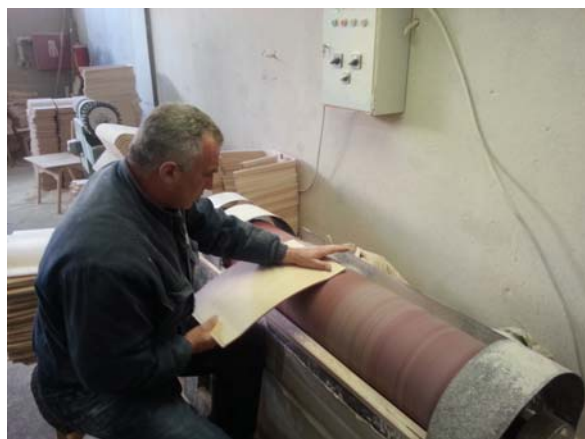
Figure 1. Processing of beech wood elements on belt grinder
