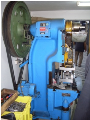
Figure 1. Eccentric press WÖGTLE (500 kN) and its frequency characteristic at individual operation
