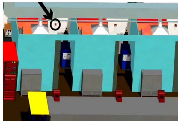
Figure 5. Single-chip computer location – 3D model of welding workplaces
