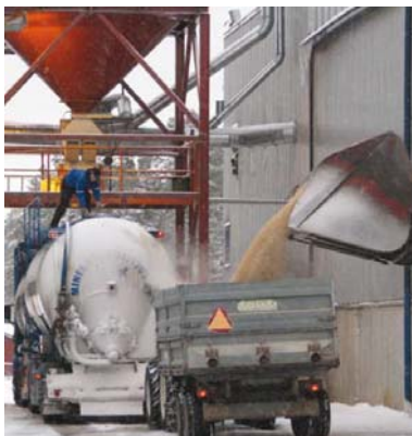
Figure 7. Simultaneous pellets loading of pneumatic truck from silo and loading of loose pellets to the tractor trailer [8]
