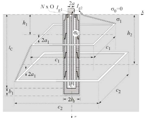
Figure 4 Pillar grounding system formed of two square-shaped electrodes.
