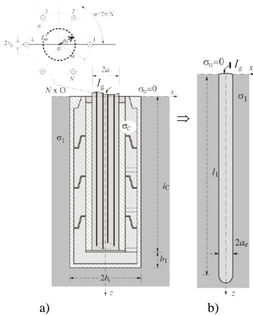
Figure 1 a) The vertical electrode system placed inside a concrete square cross-section foundation; b) An equivalent single vertical electrode placed in the homogeneous ground.
