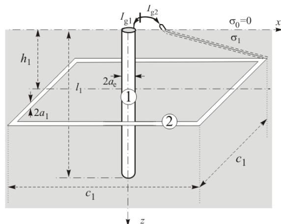
Figure 3 Equivalent system of grounding system from Figure 2.
