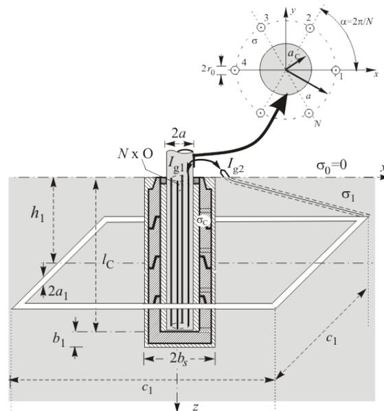
Figure 2 Pillar grounding system formed from one square-shaped electrode
