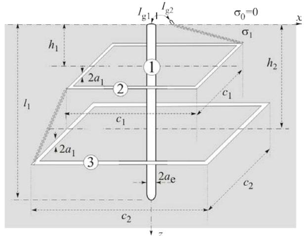
Figure 5 Equivalent system of grounding system from Figure 4.
