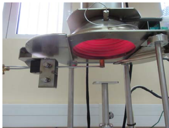
Figure 2. Instrument with a heat flux meter during the calibration phase
