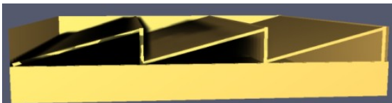
Figure 6. Smoke propagation in object with 3 slopes after 59.7 s after start with burner position at the left corner of the object
