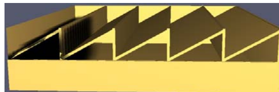
Figure 11. Smoke propagation in object with 5 slopes after 11.9 s after start with burner position at the left corner of the object
