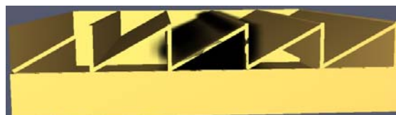
Figure 13. Smoke propagation in object with 5 slopes after 104.7 s after start with burner position at the left corner of the object
