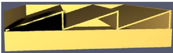
Figure 5. Smoke propagation in object with 3 slopes after 11.9 s after start with burner position at the left corner of the object
