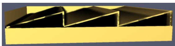
Figure 7. Smoke propagation in object with 3 slopes after 178.5 s after start with burner position at the left corner of the object
