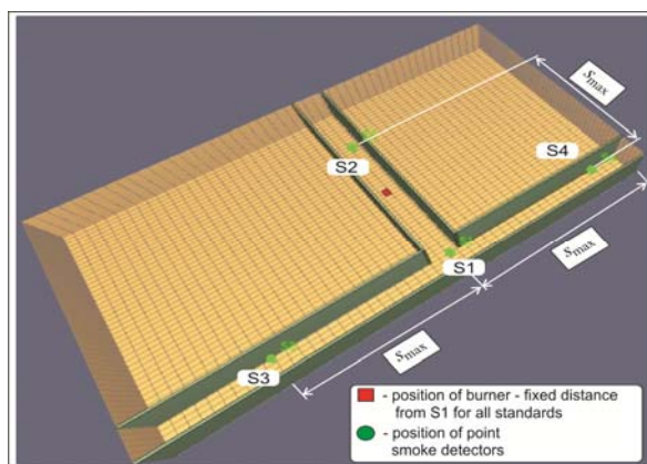
Figure 7. Simulation model with positions of burner and detectors
