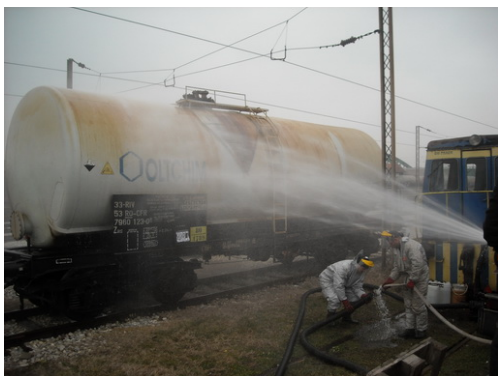
Figure 1. Emergency intervention for hydrochloric acid leak from a tank car
